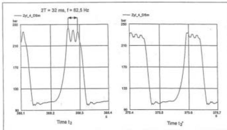
Fig. 7: Measured pressure pulsations at 330 rpm ( $t_1$ ) and 300 rpm ( $t_2$ )
