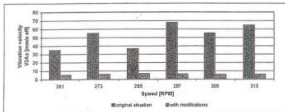
Fig. 13: Measured pipe-bend vibrations in original situation and with modification
