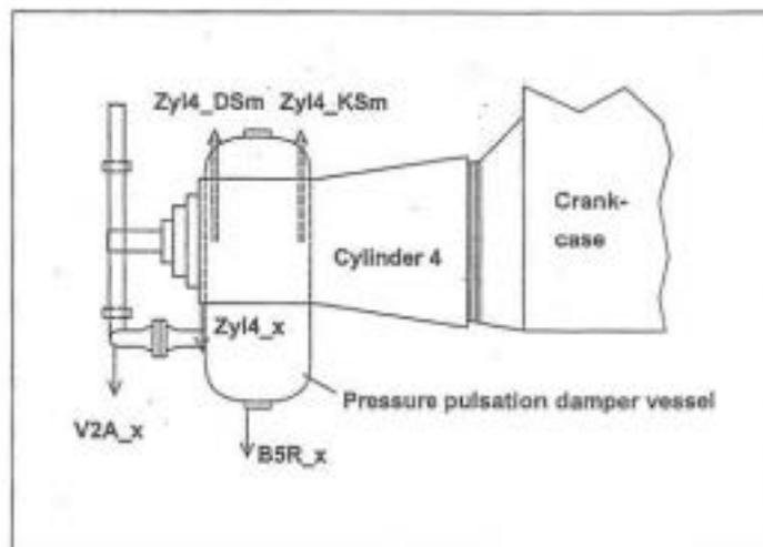
Fig. 2: Position of measurement points for detailed analysis of vibrations at Cylinder 4
