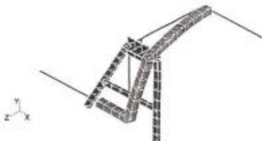
Fig. 12: FE model with 'A' support and elastomer, first natural bending frequency 79.4 Hz.
