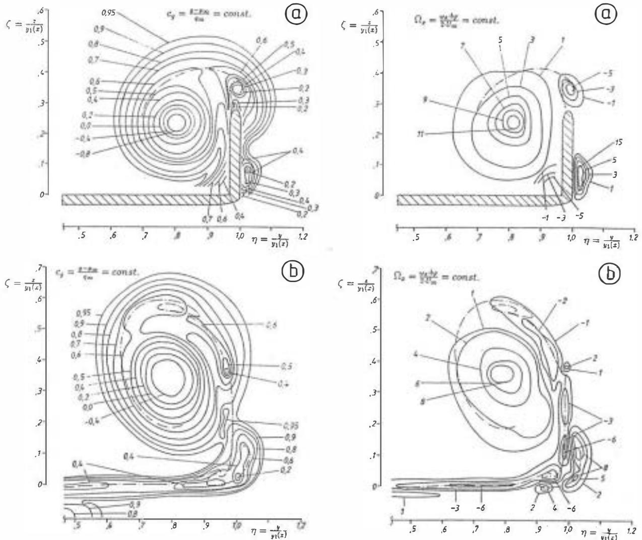
**Fig. 18:** Flowfield on the wing-fin configuration ST at  $\alpha = 13.5^\circ$ ,  $\beta = 0^\circ$  in cross-sections at a)  $\xi = 0.85$  and b)  $\xi = 1.01$ . Lines of constant axial vorticity righthand. and lines of constant total pressure lefthand.
