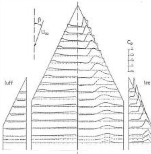
Fig. 8: Pressure distribution on the wing-fin configuration MC at  $\alpha = 10^\circ$ ,  $\beta = 20^\circ$ .
