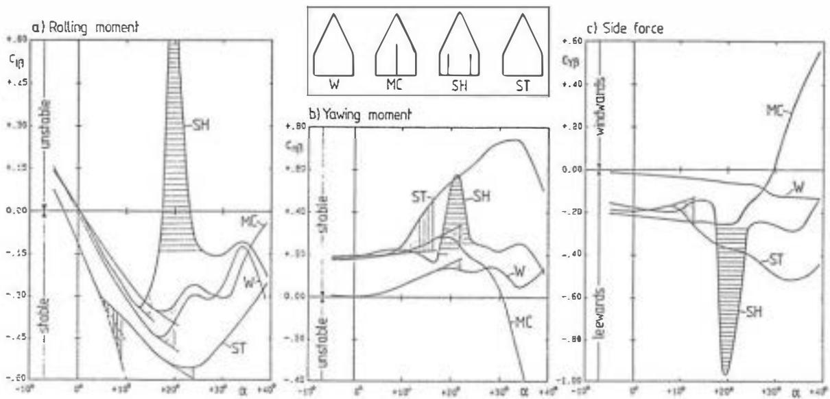
Fig. 6: Stability derivatives of the lateral motion for the wing alone W and the wing-fin configurations MC, SH, ST. Fine vertical hatching: effect of vortex breakdown, coarse vertical hatching: effect of fin vortex formation, horizontal hatching: region of high instability.
