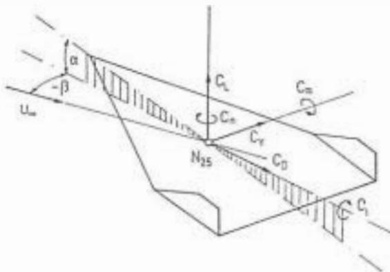
Fig. 4: Experimental coordinate system for windtunnel data reduction.
