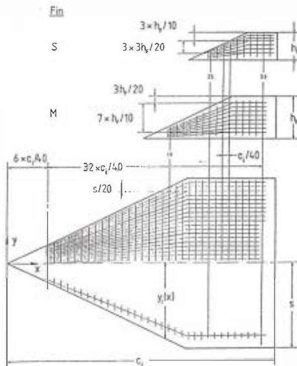
Fig. 3: Positions of the pressure taps on the wing and on the fins M and S.
