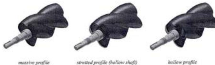
**Figure 6. Rotor profiles with different moments of inertia**
