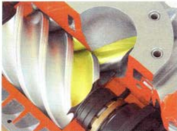
Fig. 1: Sectional representation of a screw-type motor
