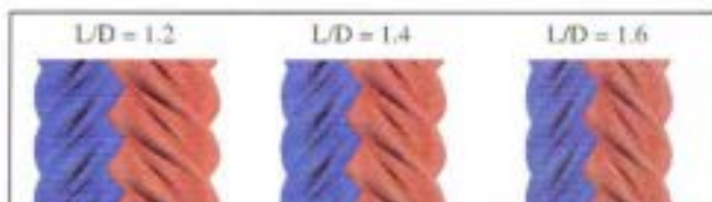
Fig. 12: Rotor pairs with differing length-diameter ratios
