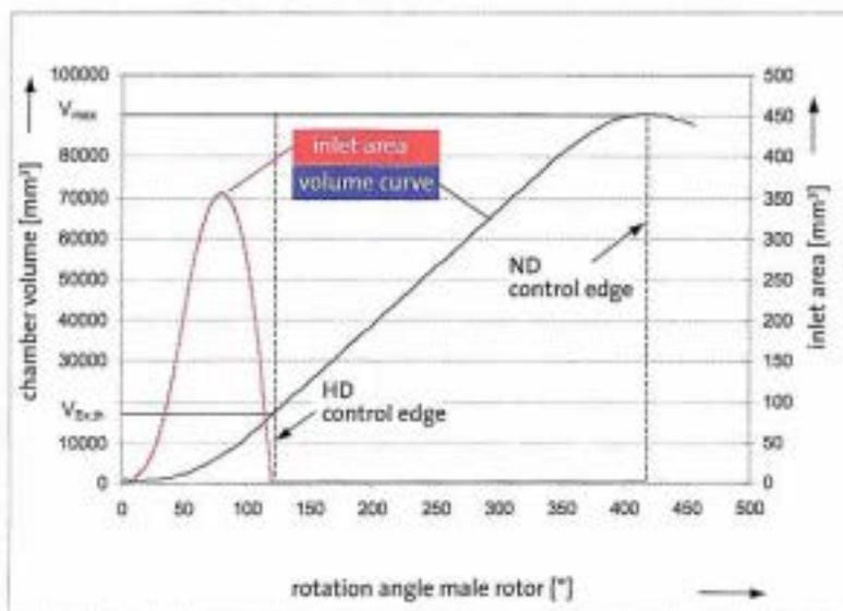
Fig.1: Inlet area and volume curve over the rotation angle of the male rotor of an exemplary screw-type engine [6]
