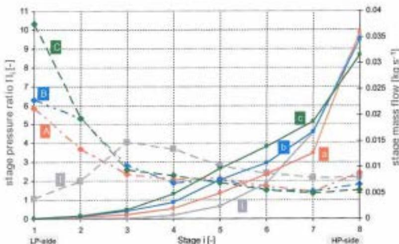
**Fig. 3.** Stage pressure ratios  $\Pi_i$  and mass flows  $\dot{m}_{C,i}$  along the rotor stages for: A: Stage pressure ratios model A; B: Stage pressure ratios model B; C: Stage pressure ratios model C; i: Stage pressure ratios isochoric rotor; a: Mass flows model A; b: Mass flows model B; c: Mass flows model C; i: Mass flows isochoric rotor.
