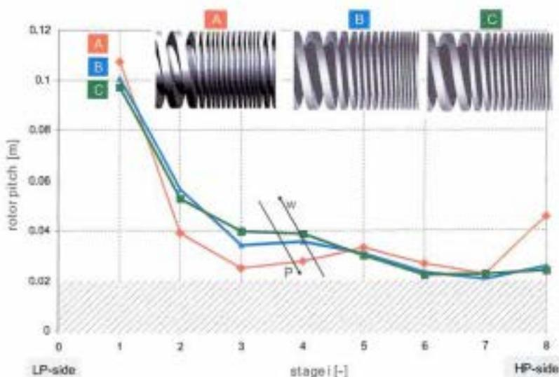
**Fig. 2.** Comparison of pitch curves for three optimized geometries selected from the Pareto-front, see Fig. 1.
