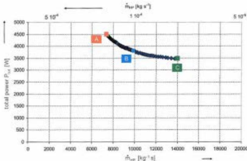
Fig. 1. Optimized total internal power and discharge mass flow shown as Pareto-front after 100 evolution steps with three selected models.
