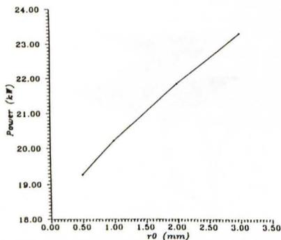
Fig. 4. Variation of compressor power with the tip radius
