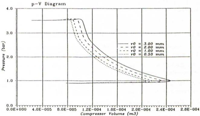
Fig. 9. Indicator diagrams for four values of the gate rotor tip radius
