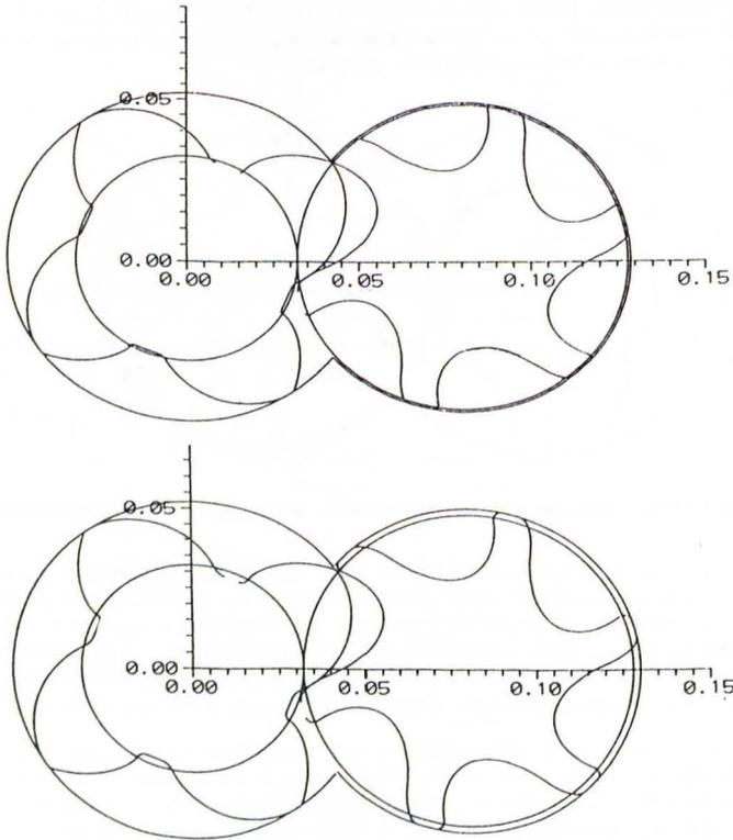
Fig. 2. Rotor pairs with new profiles for two different gate rotor tip radii
