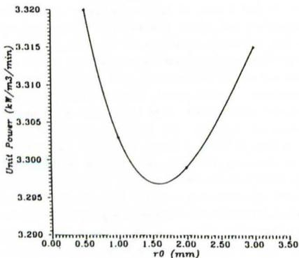
Fig. 6. Variation of unit power with the tip radius
