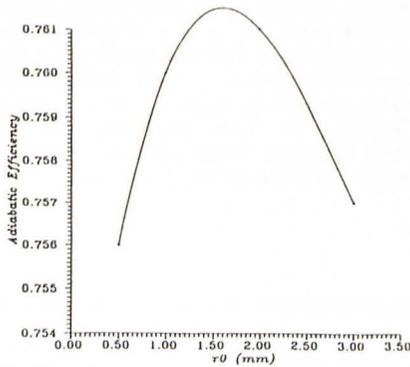
Fig. 7. Variation of the compressor adiabatic efficiency with the tip radius
