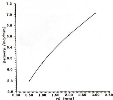
Fig. 5. Variation of compressor delivery rate with the tip radius
