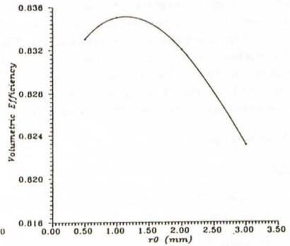
Fig. 8. Variation of the compressor volumetric efficiency with the tip radius
