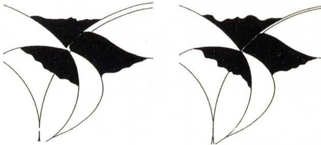
Fig. 3. A close look at the rotor tips with two different tip radii, showing the blow-hole area
