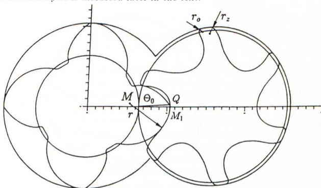
Fig. 1. Compressor rotor pair with new lobe profiles: the optimization parameters are denoted
