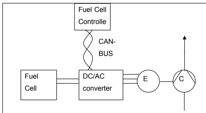
Figure 7: Schematic electric implementation of the air module components
