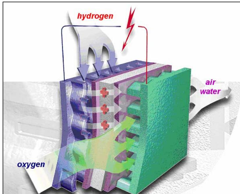
Figure 1: Basic structure of a PEM fuel cell
