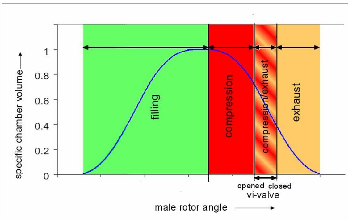
Figure 6: Volume curve for the compressor with a built-in vi-valve
