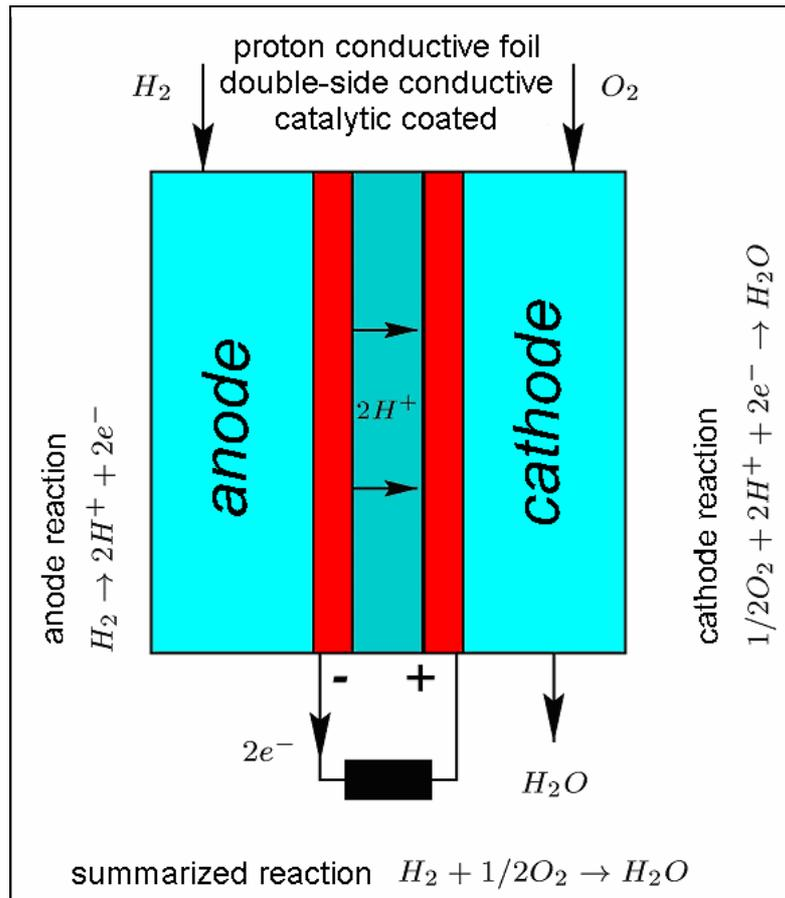
Figure 2: Chemical reactions in a PEM fuel cell [1]
