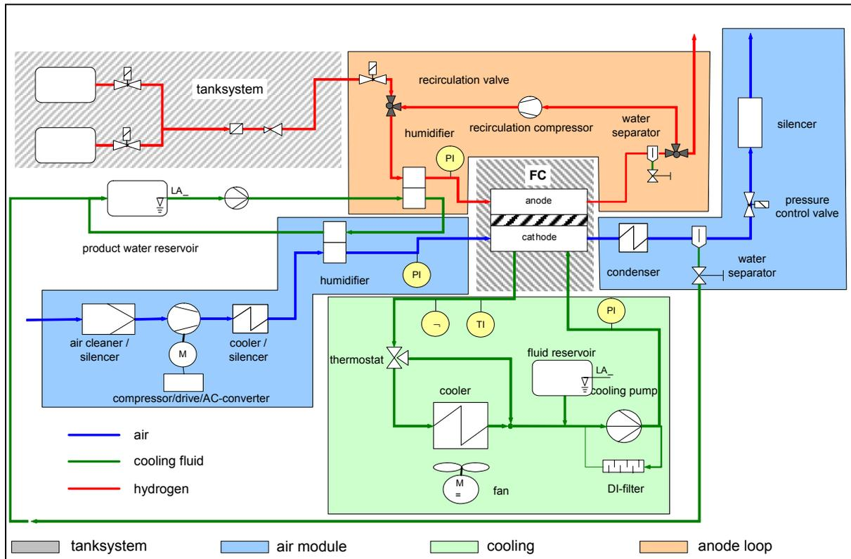
Figure 3: Schematic layout of a fuel cell system with main flow paths
