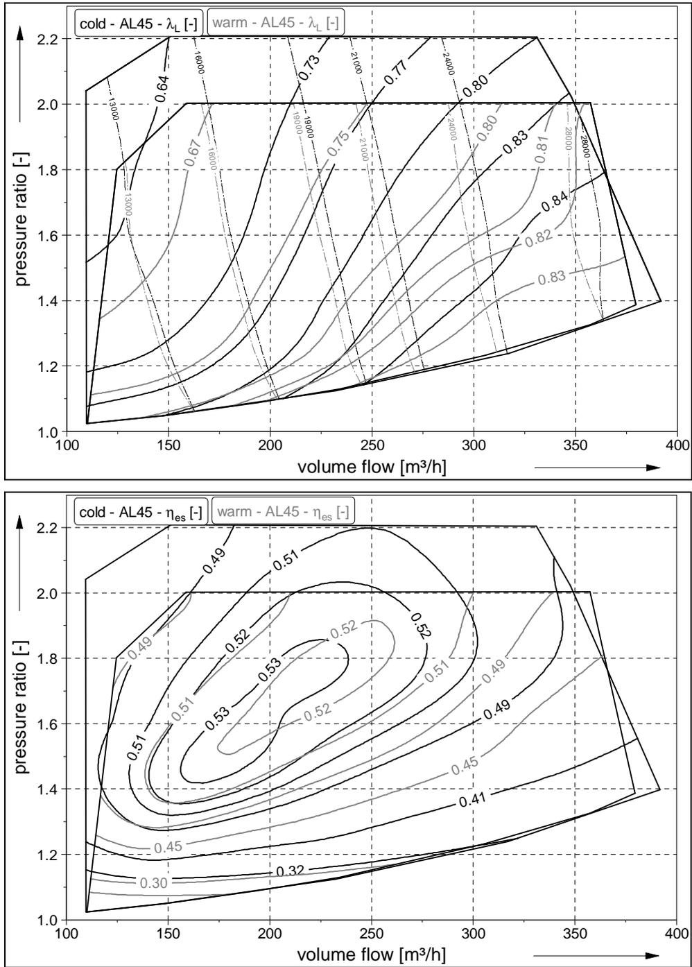
Fig. 4: Steady state and quasi-steady state volumetric efficiency (above) and effective, isentropic efficiency (below), plus male rotor speed
