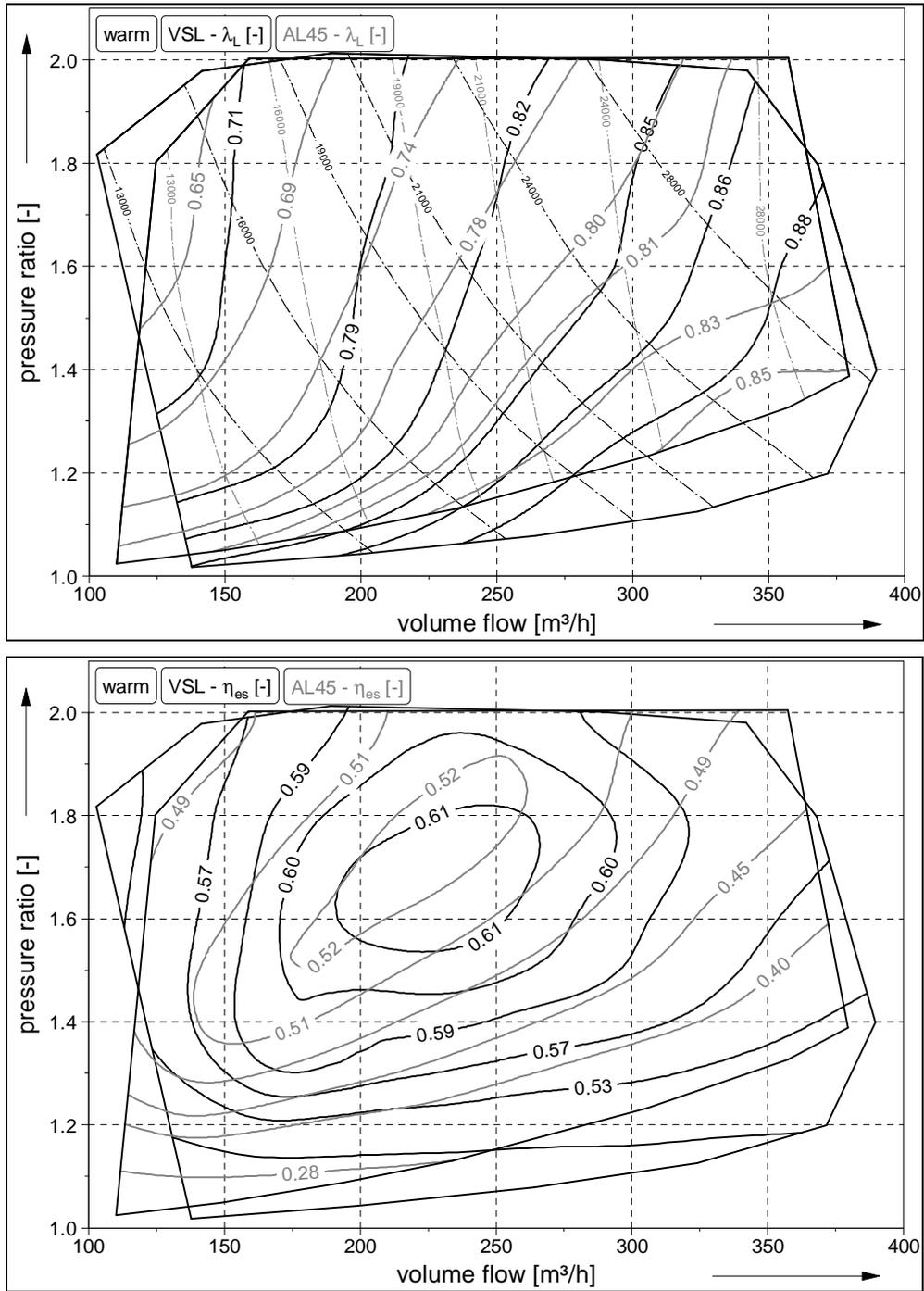
Fig. 5: Efficiency factor at steady state (above) and effective isentropic efficiency factor (below) for the screw compressor AL45 and the control screw compressor VSL. Initial conditions:  $940 < p_{in} [\text{mbar}] < 1020$ ,  $19 < \vartheta_{in} [^{\circ}\text{C}] < 22$ , Dotted lines (male rotor speed, in  $\text{min}^{-1}$ ),
