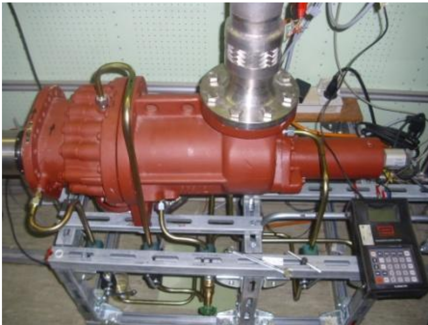
Fig. 3: Screw machine Aerzen Variscrew VMY 046 HR V_N : 1,04 m 3 /min at 3025 min -1
