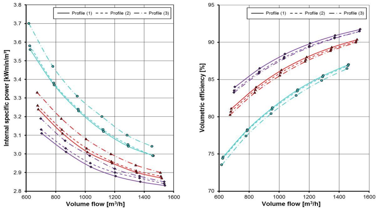
Fig. 6: Specific power and volumetric efficiency over volume flow at 3.5 bar (abs.)
