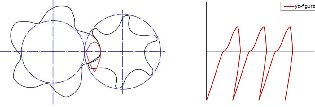
Fig. 1c: Based on Kaeser Sigma Profile (3)
