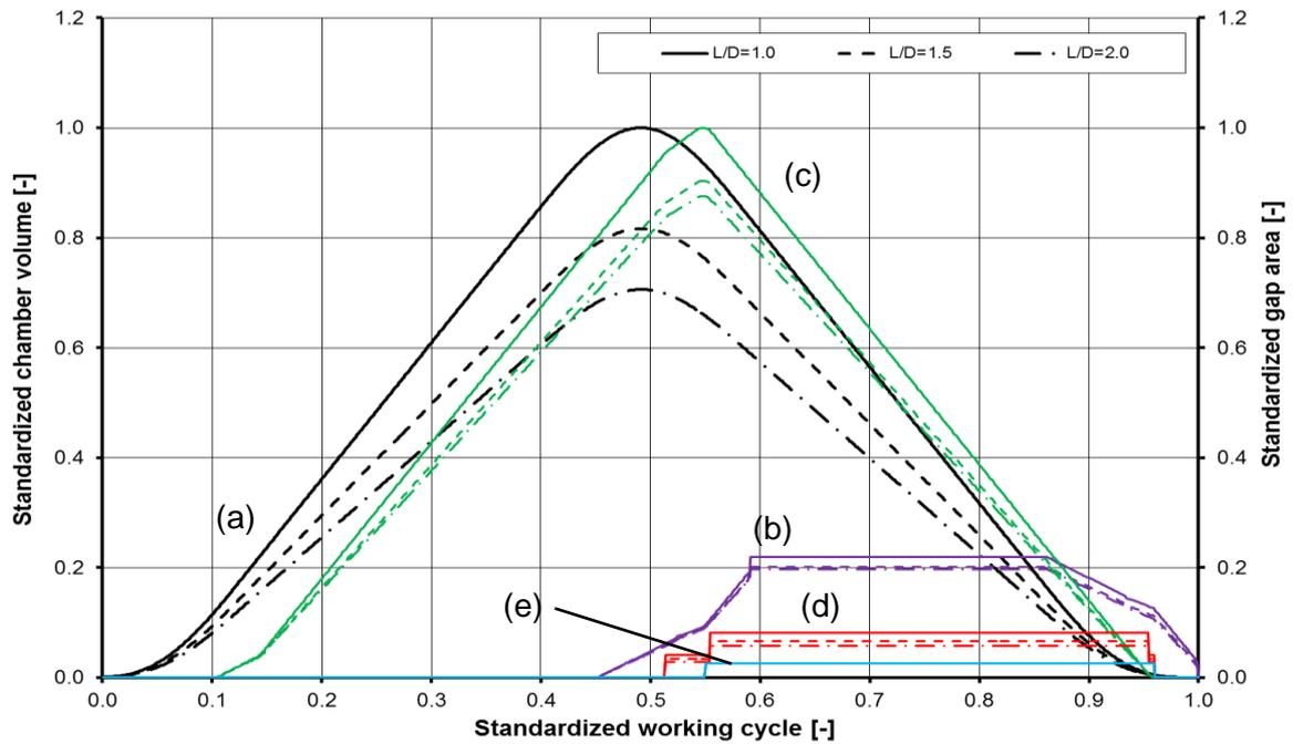
Fig. 5: Influence of length over diameter ratio from 1.0 – 2.0
