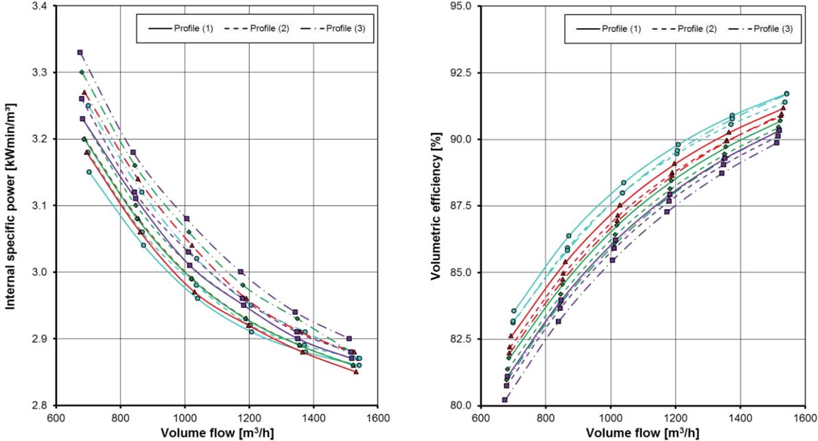
Fig. 8: Specific power and volumetric efficiency over volume flow at 3.5 bar (abs.)
