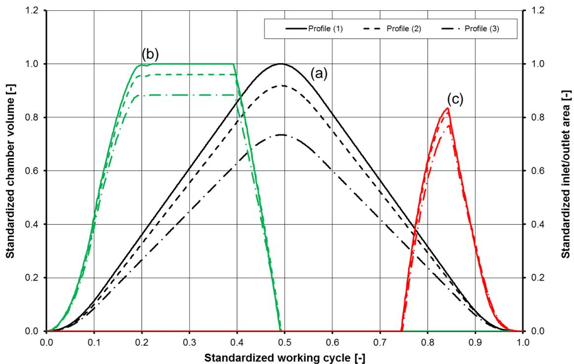
Fig. 3: Standardized volume (a), inlet (b) and outlet (c) curves at same center distance
