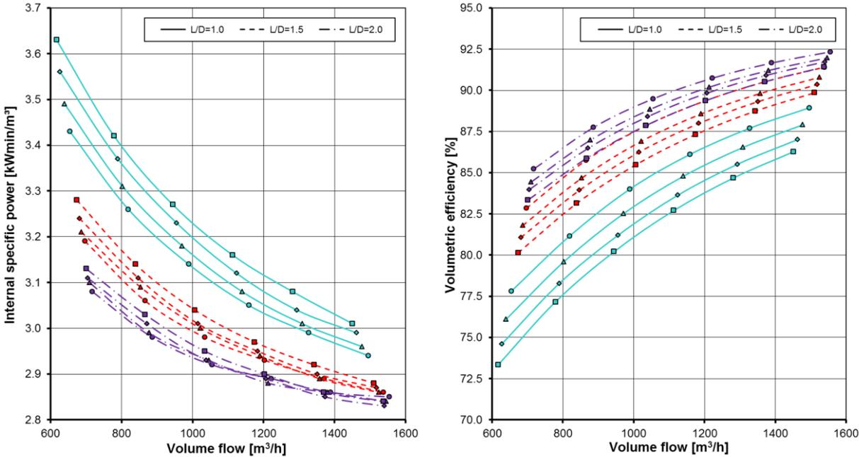
Fig. 9: Specific power and volumetric efficiency over volume flow at 3.5 bar (abs.)
