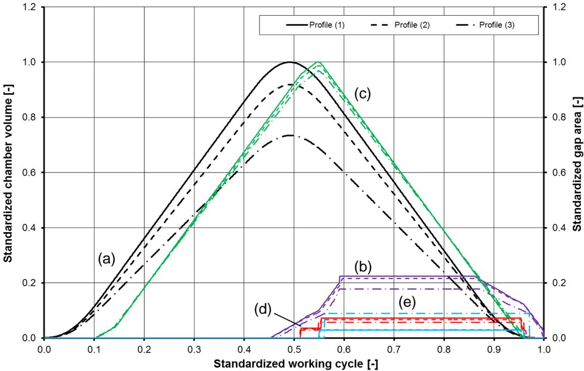
Fig. 4: Standardized volume and gap area curves at same center distance
