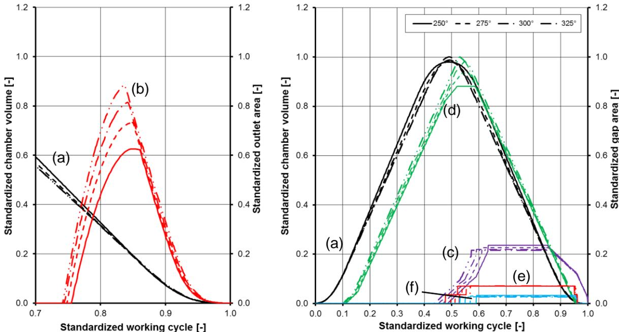
Fig. 7: Influence of male rotor wrap ( $\varphi_{MR}$ ) angle from 250-325°
