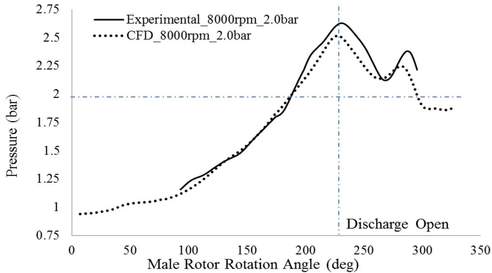
Fig. 3 Pressure-angle diagram obtained by CFD and Measurements
