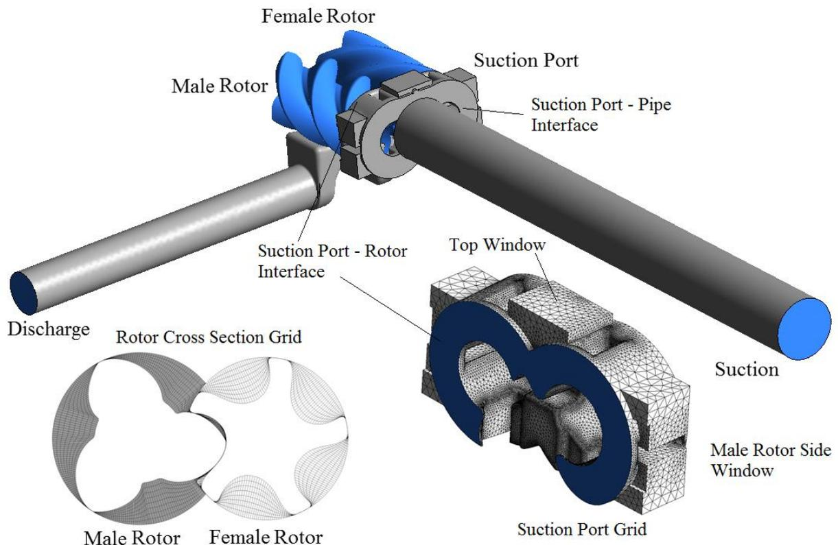
Fig. 2 Full 3D model for analysis of the single phase flow in the test screw compressor
