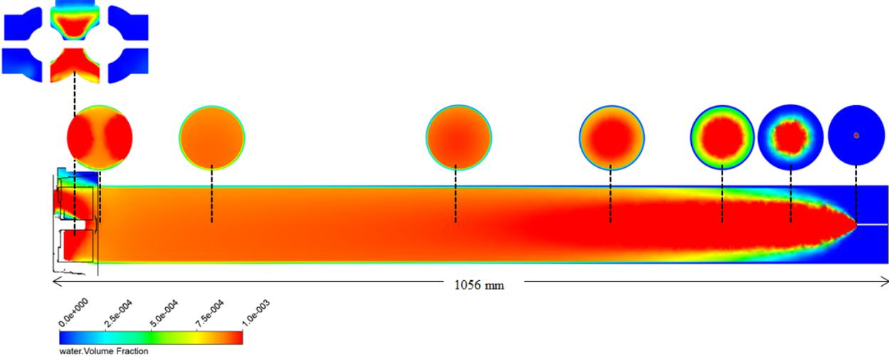
Fig. 9 Volume fraction of water across the pipe and suction port
