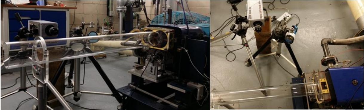
Fig. 4 Experimental setup for testing and visualisation of suction flow
