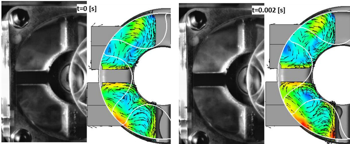
Fig. 5 High speed camera and CFD comparison for the gate rotor
