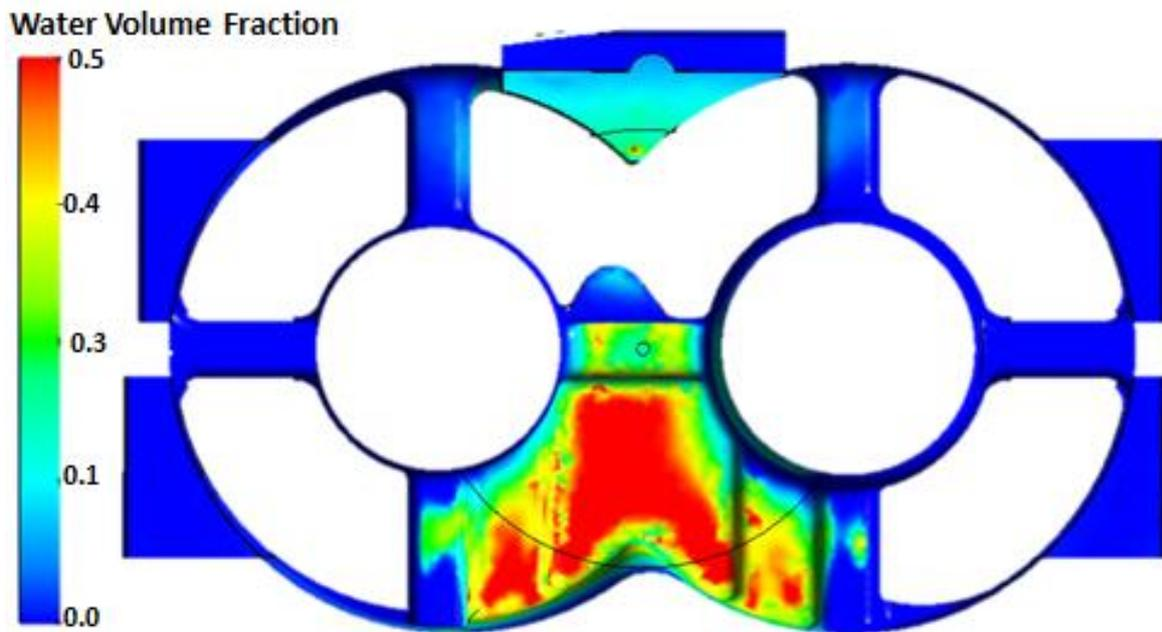
Fig. 10: Water depositions on the surface of the suction port
