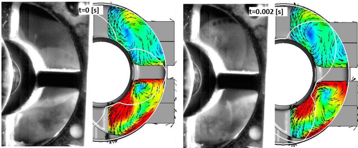
Fig. 6 High speed camera and CFD comparison for the male rotor
