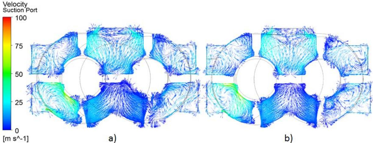
Fig. 8 Velocity vector plot at the suction a) Full case b) Suction port model
