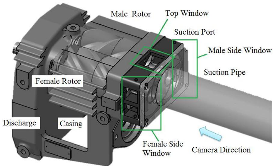
Fig. 1 Screw compressor with Suction port windows and extended suction pipe
