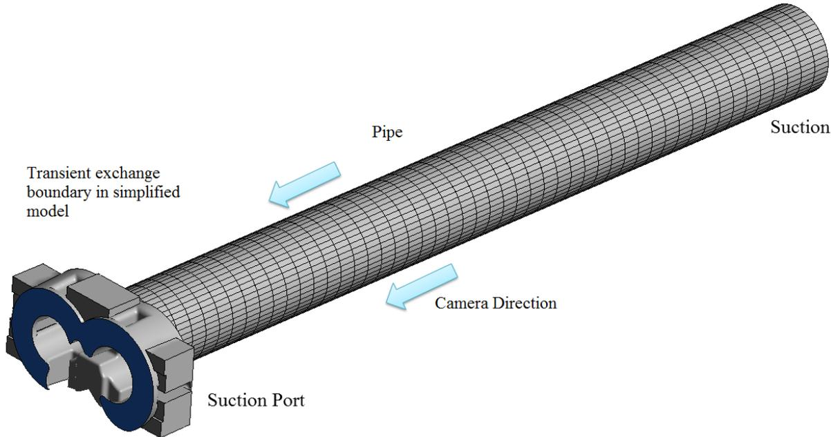
Fig. 7 Reduced Multiphase CFD model with the transient boundary interfacing with rotors
