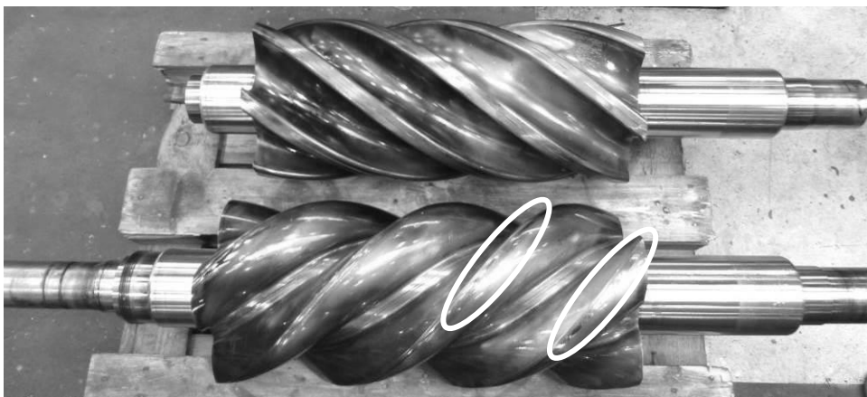
Fig. 14: Wear on male and female rotor due to contact with slide valve
