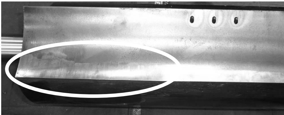
Fig. 13: Wear on slide valve due to contact with male and female rotor
