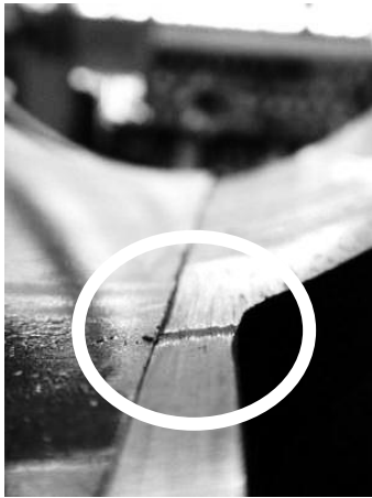
Fig. 9: Detail Slide valve scuffing
