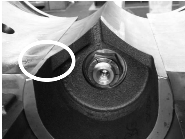
Fig. 10: Slide Valve scuffing
