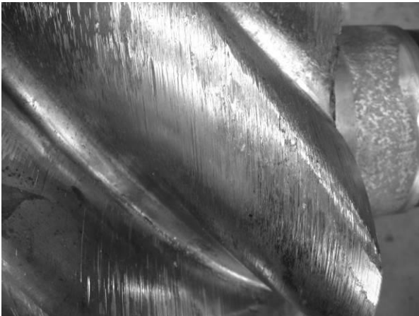
Fig. 7 Wear (male rotor) due to liquid carryover
