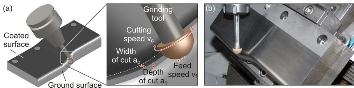
Fig. 3: NC grinding on machining centres using spherically shaped mounted points. (a) Process kinematics and (b) picture of the grinding process
