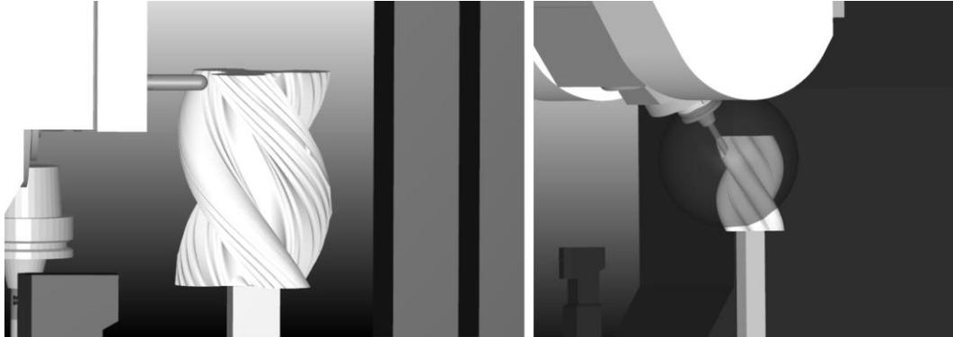
Fig. 2: Virtual Machine with removed material (left) and detected surface collision (right)
