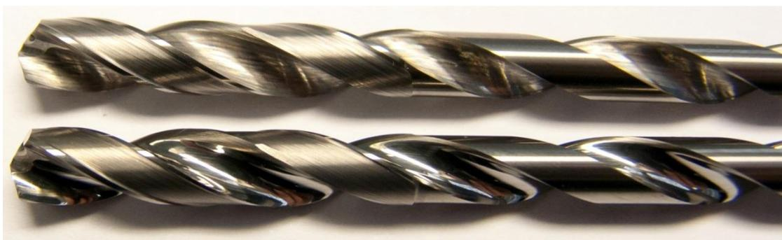
Fig. 7: Comparison between ground and polished drill flute of a solid carbide tool
