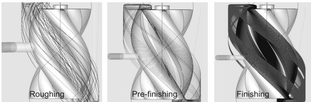
Fig. 1: Disparity of generated NC-paths for different operation steps
