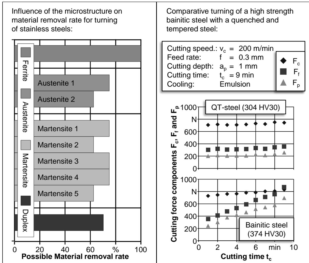
Fig. 4: Examples of material influence for machining of difficult to cut steels ( $F_c$ =cutting force,  $F_f$ =feed force,  $F_p$ =passive force)
