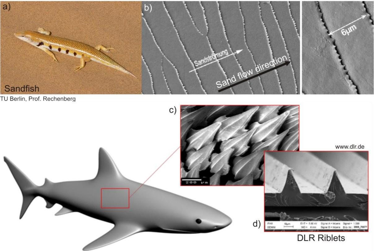
Fig. 5: Scanning electron microscope recordings of sandfish skin (b) [12], sharp skin structures and the DLR Riblets [15]
