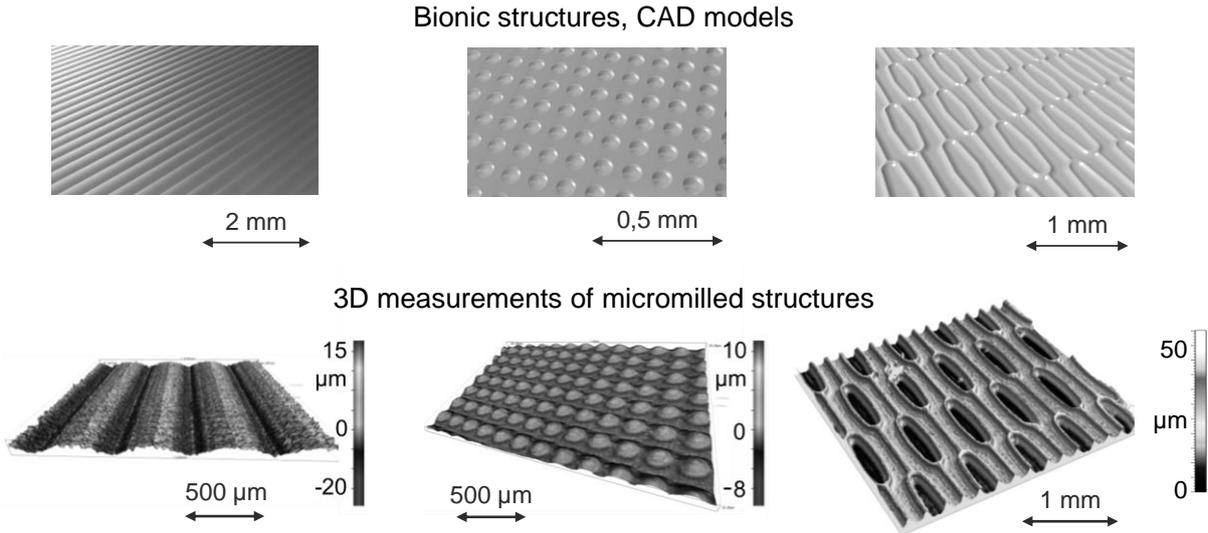
Fig. 6: Overview of some CAD models and machined surfaces from bionic structures (beetles)
