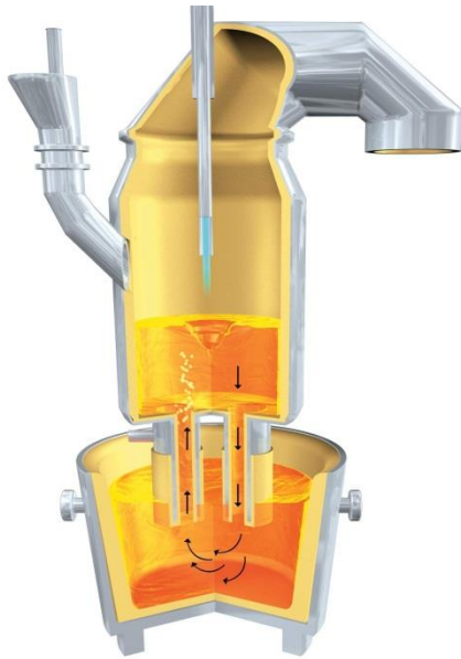
Fig. 3: Ruhrstahl-Heraeus (RH) steel degasser, works graphic Oerlikon Leybold Vacuum
